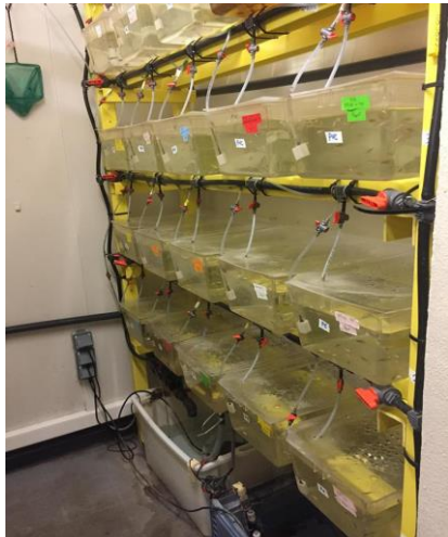
Automated flow-through system with 30% of daily water renewal
